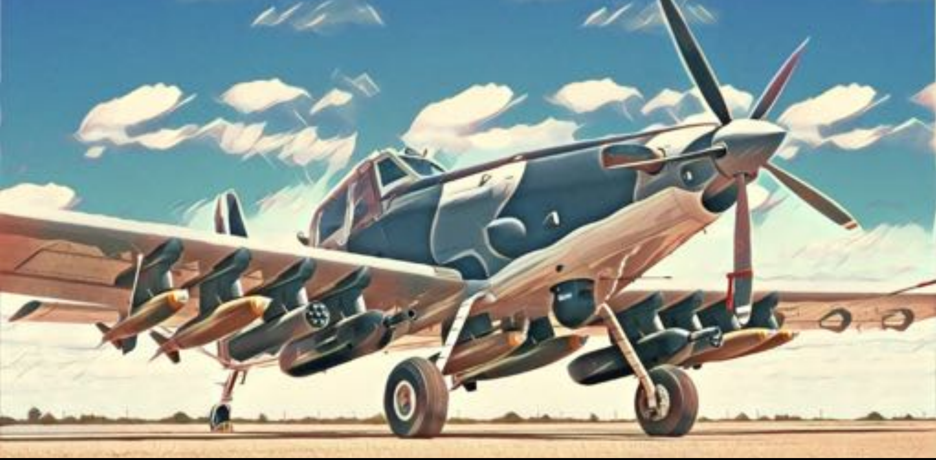
In response to the United States Air Force's LAAR program and the growing requirement for light counter-insurgency aircraft, Air Tractor developed an armed model, the AT-802U , in 2008, with engine and cockpit armor, a bulletproof windscreen, self-sealing fuel tanks, and structural reinforcements for the carriage of 9,000 pounds of payload.
