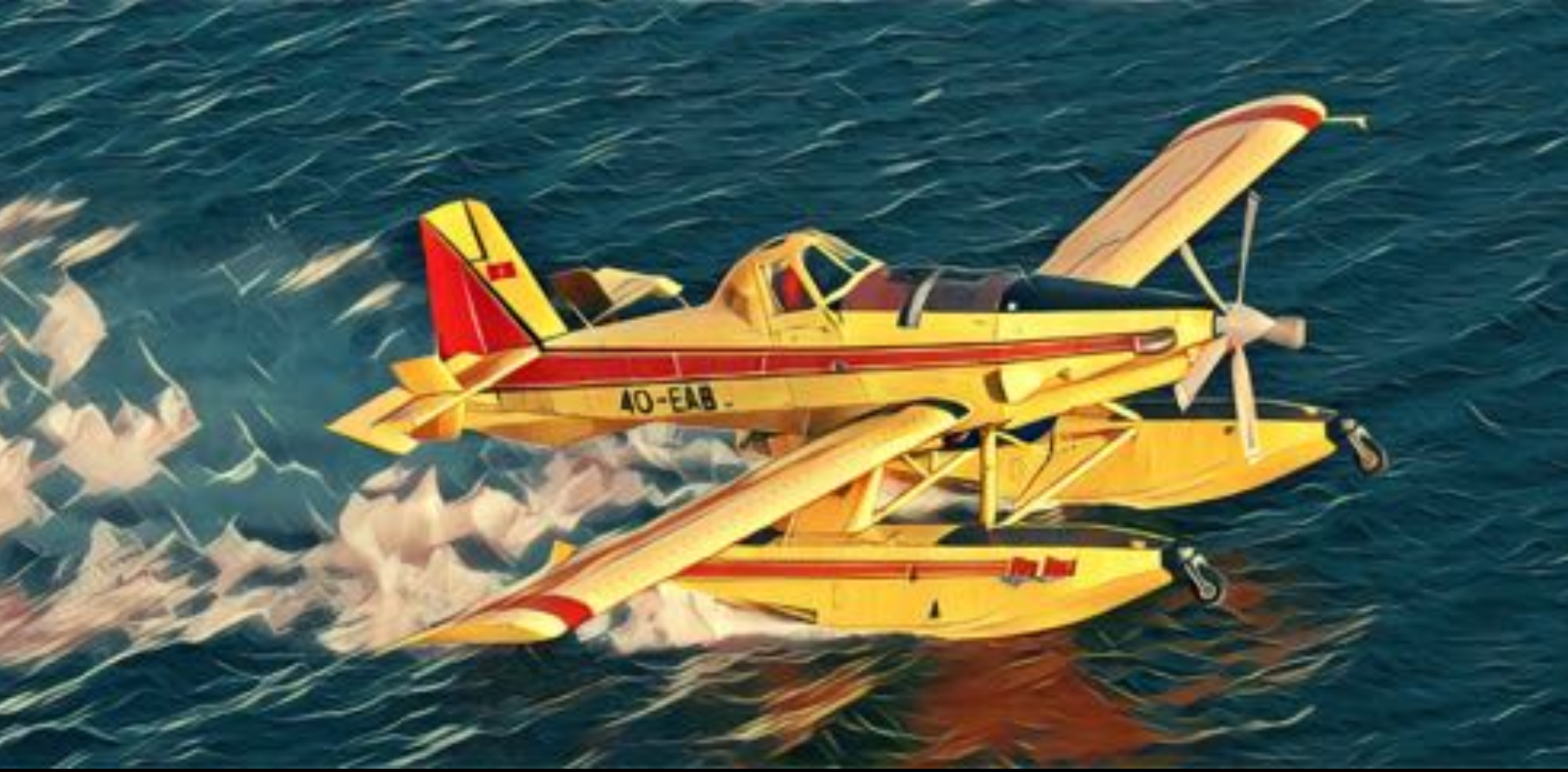
The Air Tractor AT-802 Fire Boss is an agricultural aircraft that may also be adapted into fire-fighting or armed versions. It first flew in the United States in October 1990 and is manufactured by Air Tractor Inc. A number of aircraft have been converted to the Fire Boss aerial firefighting configuration, which utilizes Wipaire 10000 amphibious floats, so that it can land on a traditional runway or on water. The Fire Boss can scoop water from a lake or river for use on a fire.
